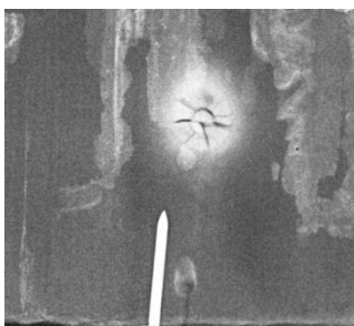
Fig. 149. Detail Rx. It is noted nail from the wood, metal pin and node concrescent
